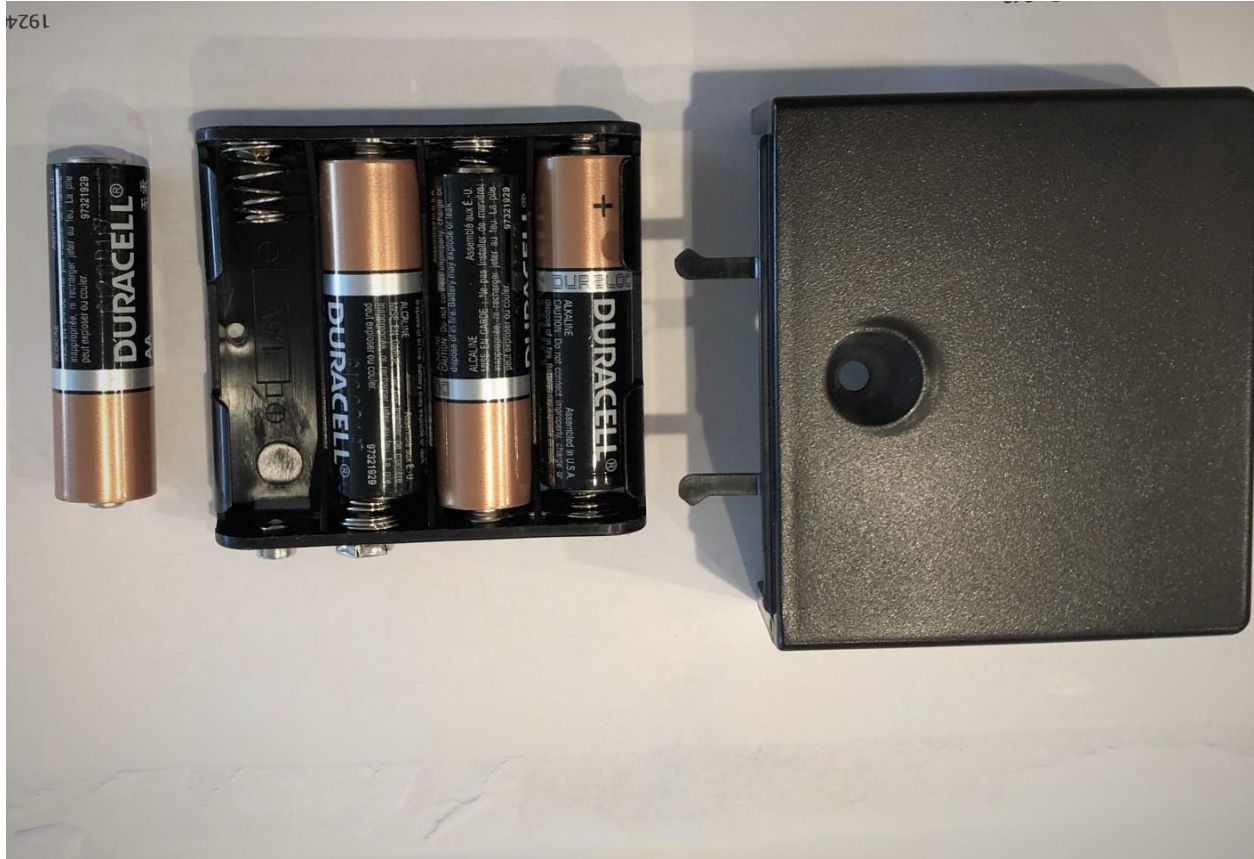
Figure 1: Battery pack, removed from lock. 4 AA batteries needed. Install with the correct polarity! Recommended change interval one year
